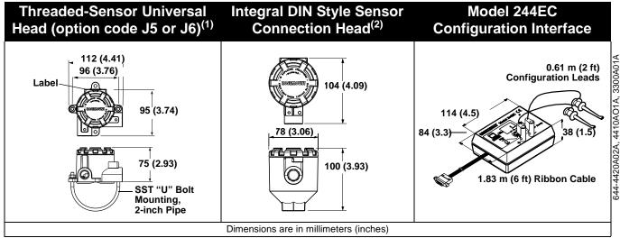
(1) A "U" Bolt is shipped with each universal head unless assembly option code X1, X2, or X3 is ordered.
